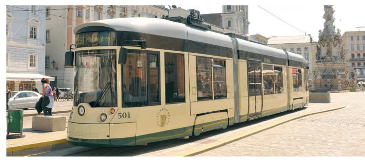
Linz Linien ordered three 100% low-floor trams, based on the proven *BOMBARDIER\* FLEXITY\** Outlook concept. The vehicles are designed for operation on the historic track to the top of the Pöstlingberg Mountain in Linz, Europe's steepest tram line. Accordingly, the trams feature a nostalgic design consistent with the existing historic vehicles.
